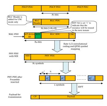
Fig. 7. PUSSCH Payload Transmission Format
