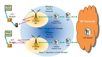
Fig. 2. IoT Wide Area Communication System: Initial Setup and Operation
