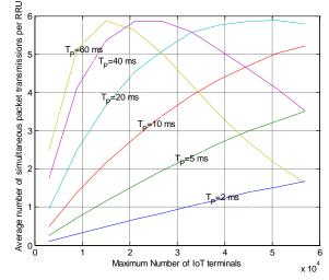
Fig. 9. Performance of the simultaneous access contention mechanism
