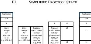
Fig. 4. Protocol Stack for IoT Air Interface
