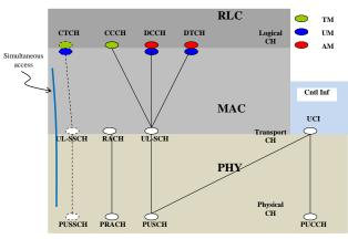
Fig. 6. Channel mapping for IoT Air Interface
