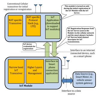
Fig. 1. RAT agnostic IoT Module for Wide Area Communication System
