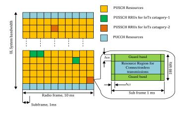
Fig. 5. Radio Resource Grants for ULSSCH IoT Transmissions in a 10 MHz LTE Uplink Band
