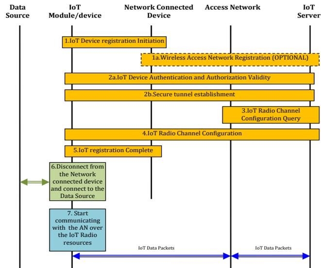
Fig. 3. IoT Module Setup Procedure
