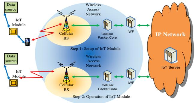
Fig. 2. IoT Wide Area Communication System: Initial Setup and Operation
