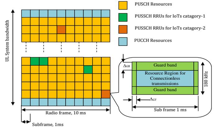
Fig. 5. Radio Resource Grants for ULSSCH IoT Transmissions in a 10 MHz LTE Uplink Band
