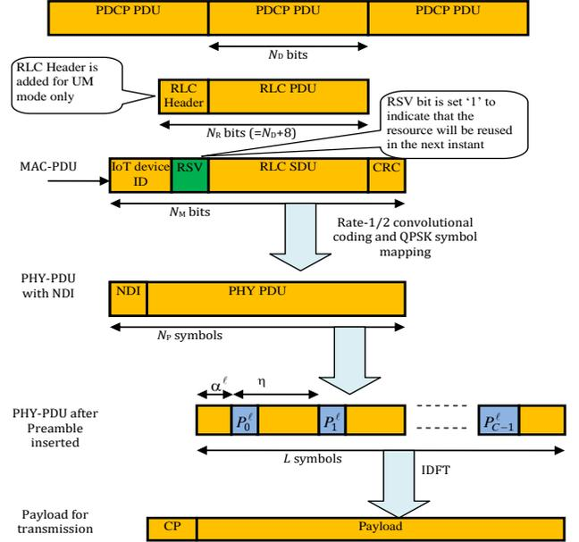
Fig. 7. PUSCH Payload Transmission Format
