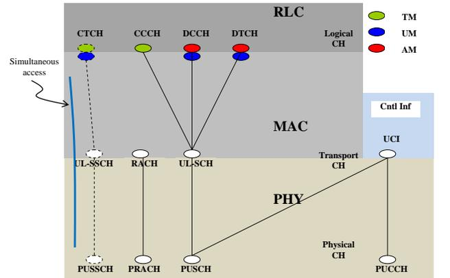
Fig. 6. Channel mapping for IoT Air Interface
