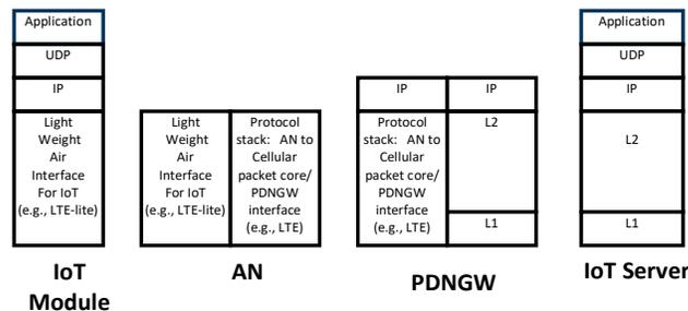
Fig. 4. Protocol Stack for IoT Air Interface
