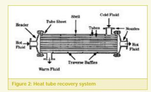
In this situation the boiler makeup water would be passed through the cold fluid line and the process fluid would be passed through the hot fluid line. The energy performance of the shell and tube type of heat exchanger depends on the application, but may be as high as 80–90%. Shell and tube heat recovery units can be designed to manage most operating conditions and temperatures up to 500°C.
