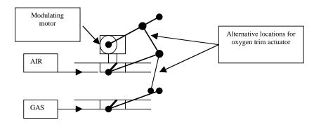
Figure 2: Linked valve air–gas ratio control
