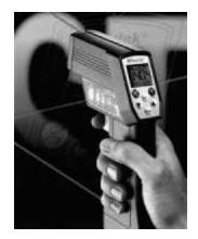
**Figure 9. Infrared temperature gun.** (Illustration courtesy of Raytek Corporation)
