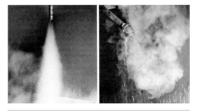
Figure 6. Live steam versus flash steam. (Illustration courtesy of Yarway Corporation)
