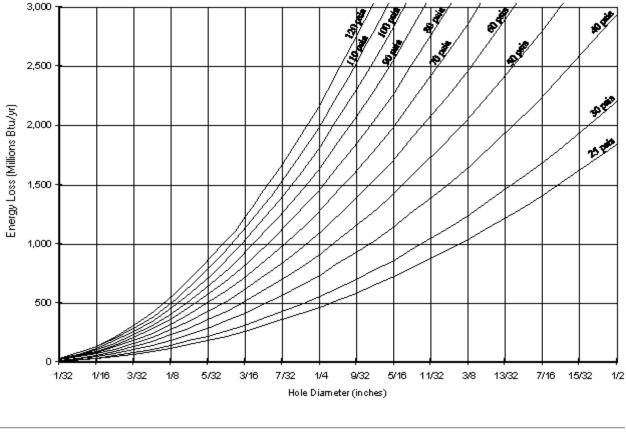
Figure 10. Energy loss from leaking steam traps.
