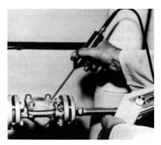
**Figure 8. Ultrasonic test kit.** (Illustration courtesy of GESTRA, Inc.)
