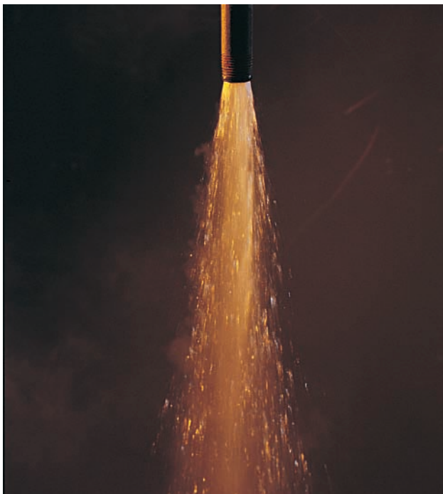
Fig. 4—To determine trap performance by visual observation of condensate discharge, you should know the difference between flash steam (lazy vapor discharging with condensate—left) and live steam (high temperature, high velocity discharge—right).
