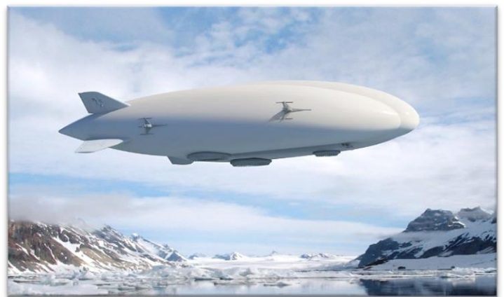
Lockheed Martin's Hybrid Airships will be used to transport ~100,000 tonnes per year of concentrate from Strange Lake
