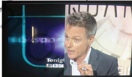
Off screen shot of Lo23's mixer back in action- a horizontal wipe between rather random source material; a BBC Scotland news promo graphic (on the Picturebox) and a VT playback of a tape I found in the truck, a rehearsal for a 'Culture Show' OB from around 2010.
