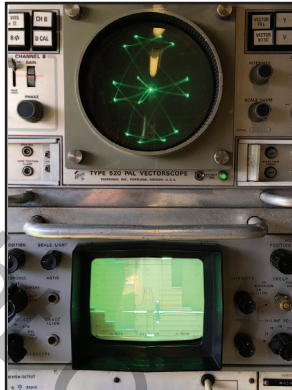
If the camera colour bars look like this, then all is well. If the burst timing (the 90 deg. angle in the centre of the vector monitor, top) is not aligned, the chroma phase is out and the PAL coder needs tweaking. There is none of this malarkey now with digital. It just works- or doesn't.
