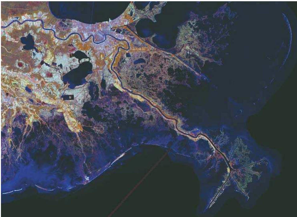
FIGURE 5.54 Satellite image showing a river-dominated, prograding delta in an overall transgressive setting (case B in Fig. 5.52; Mississippi delta, Louisiana; image released by the U.S. Geological Survey National Wetlands Research Center). The high sediment supply of the river causes the delta to prograde in spite of the transgression recorded by the adjacent open shorelines.
