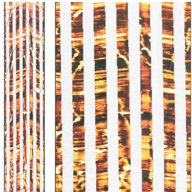
FIGURE 2.30 New micro resistivity logs combine resistivity with dipmeter data to produce 'virtual cores' in three dimensions. Such detailed borehole imaging, with a vertical resolution of less than 8 mm, allows the observation of sedimentary structures in the absence of mechanical core (modified from data provided by Baker Atlas).
