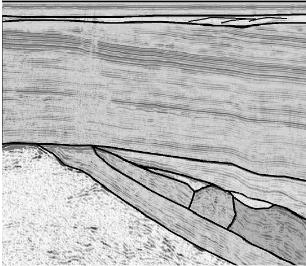
Fig. 14. [Reproduced in colour in Plate 3 on page 422.] Overlay of different colours onto the same inline as for Figure 13. This represents a vision how a seismic data set should be segmented into shapes and textures. Different colours correspond to different shapes and textures. Compare Figure 13 for legend.
