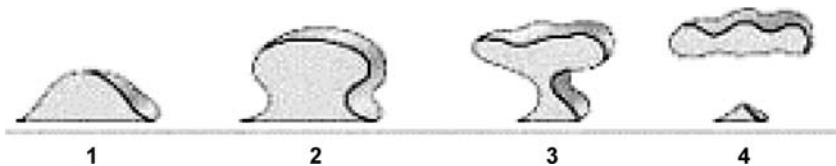
Fig. 14. Illustration of the evolution of a salt diapir.
