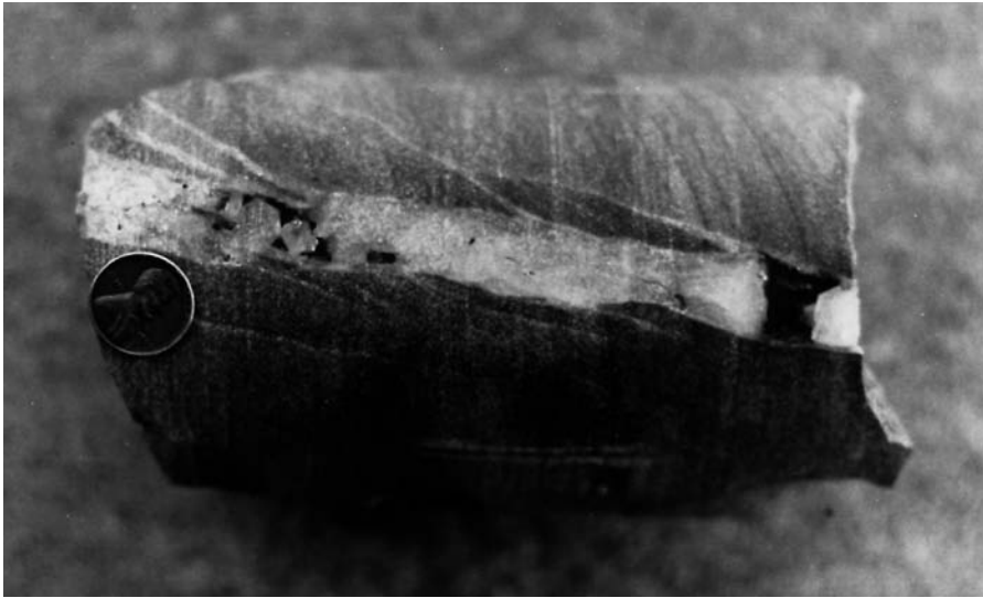
Figure 1–47 Incompletely mineralized fracture in Silurian Tuscarora Sandstone on SEM photomicrograph from the Amoco No. 1 Texas-Gulf Well, Centre County, Pennsylvania. Photo courtesy of R.E. Larese.
