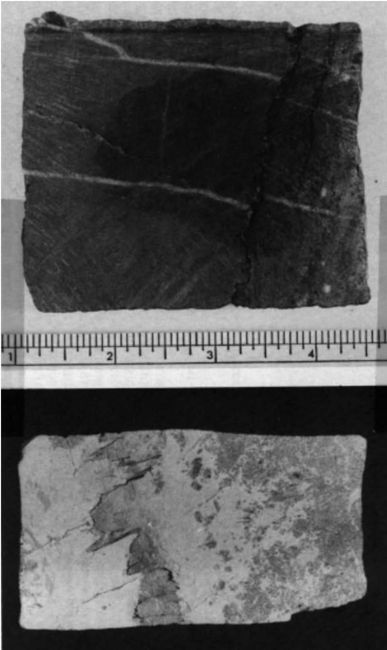
Figure 4-3 Examples of association of stylolites and tension gashes in 4-in. diameter core of Yamama Limestone, Darius Field (Wells D-3 and D-4), Persian Gulf. From Nelson (1981a), courtesy of AAPG.
