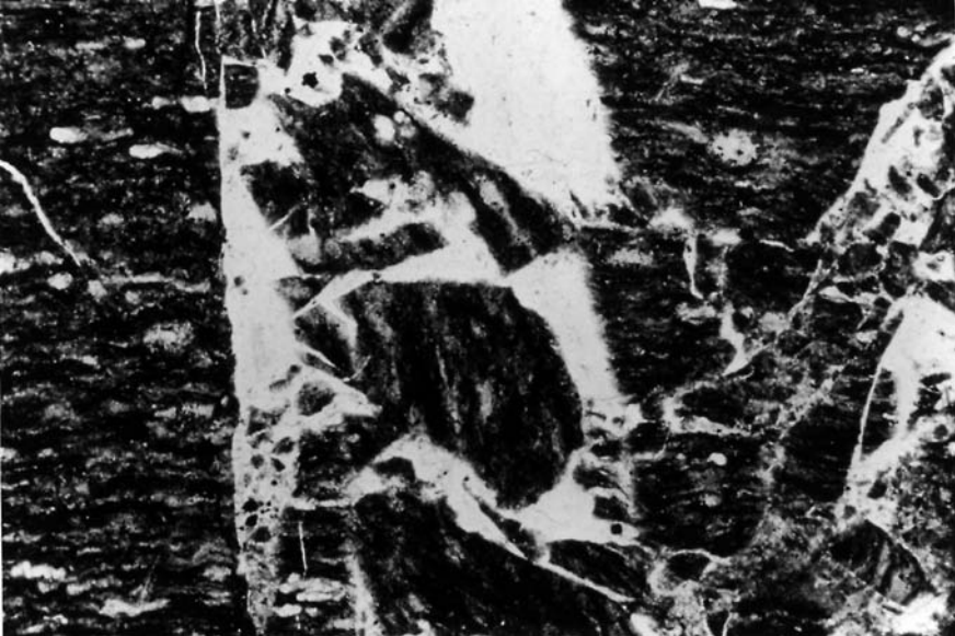
Figure 1–31 Gouge in thin section in plane (above) and polarized (below) light. Sample is Devonian Woodford shale.
