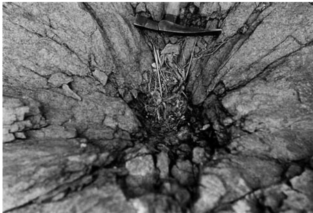
Figure 5-2 Radial blast or explosive induced fractures in outcrop, southern Oklahoma.
