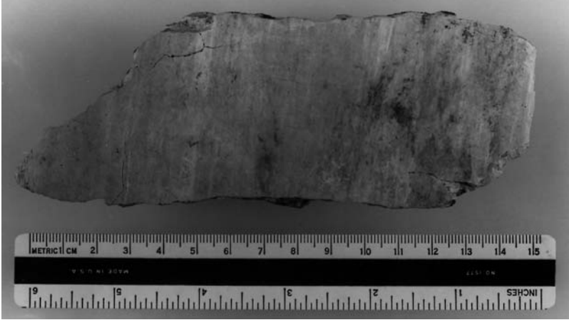
Figure 1-40 Slickensided fracture in a limestone outcrop sample from the Deer Creek Thrust, Nevada.
