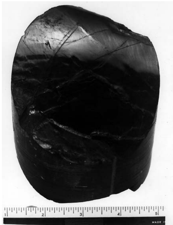
Figure 1–43 Slickensided fracture in shale. Sample is from Devonian Second White Specks, Alberta, Canada.
