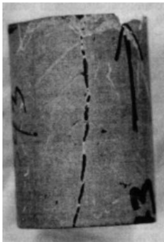
Figure 1–50 Vuggy fracture in carbonate core. Courtesy of B.J. Ward, Jr. (Magnification 1.5x.)
