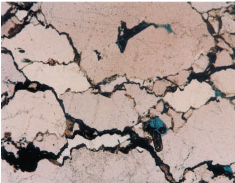
Plate 3. Thin section micrograph of an interconnecting network stylolites. Stylolites of this type are only abundant at depth greater than 2.0 km, Flacourt Formation, 2714.4 m, Griffin-1.
