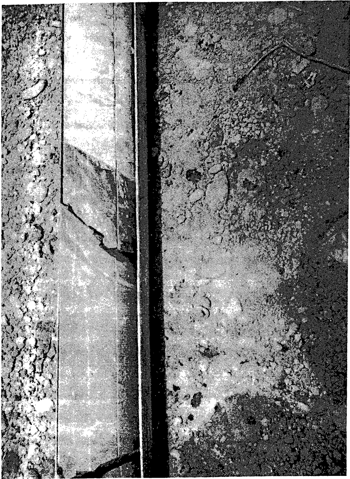
Fig. 3.16 Scribe Mark on Oriented Core
