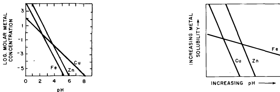
Fig. 210. Change in metal solubilities with change in pH for a solution at 250^{\circ}\text{C} , S = 10^{-3}\text{M} , \Sigma \text{Cl}^{-} = 1\text{M} , and p\text{O}_2 = 10^{-48}\text{ atm} . It can be seen that if pH was the dominant control on sulphide precipitation then orebodies would be zoned from Fe \rightarrow Zn with Cu in all zones; p\text{O}_2 = oxygen fugacity (pressure). (After Finlow-Bates, 1980.)
