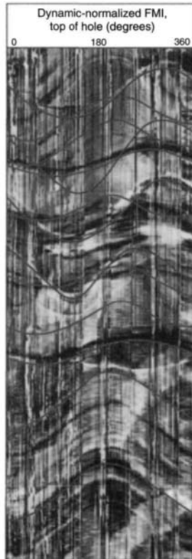
Features in whole-core image matched to equivalent features resolved by FMI data in deviated well
