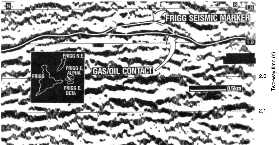
Fig.3.9 A direct hydrocarbon indicator at the gas/oil contact in the Frigg Field, North Sea. In common with other DHIs, the flat spot will be horizontal on a depth-migrated section. (From Héritier et al. 1990.)
