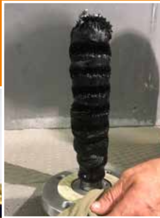
Ferro Cleaner magnet after 1 year of operation
