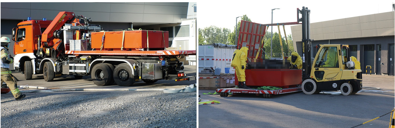
Left: With a WLF, the WF Mercedes-Benz brought a battery salvage container. right: By means of a forklift truck, the damaged battery together with the carrier frame was brought into the salvage container.
