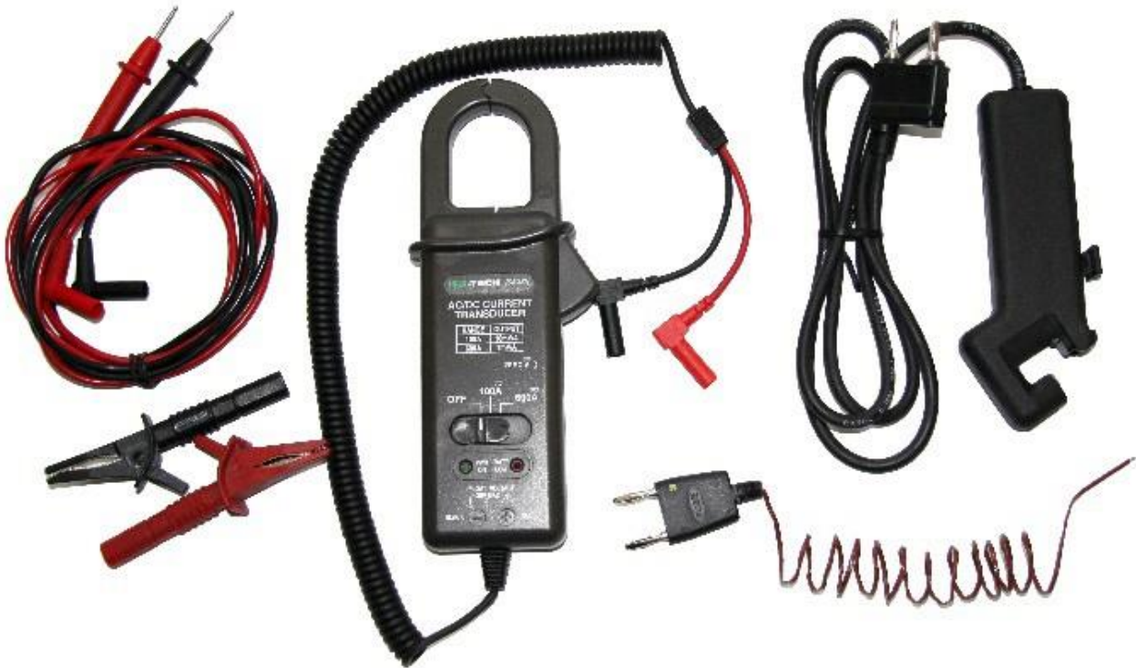
Figure 44. Fluke 78 Automotive meter and accessories (test leads, 600A clamp, plug lead RPM, temperature thermocouple)
