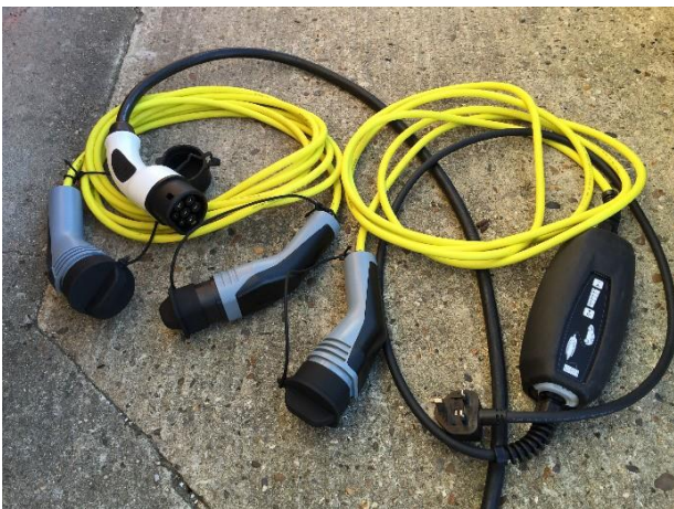
Figure 172 Domestic mains and charge point cables
