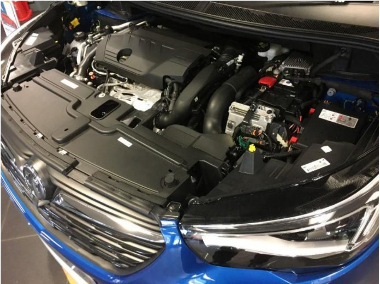
Figure 205 This is a Vauxhall Grandland hybrid – but it is hard to tell without looking very closely for the orange wires, take care!
