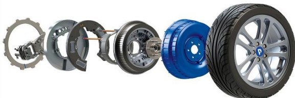
Figure 79 Protean Electric's in-wheel motor system is arguably simpler than a conventional electric automobile, which has constant-velocity joints, drive shafts, and a centrally mounted transmission and motor (Source: Protean Electric)
