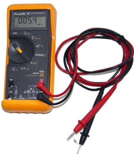
Figure 48. Checking a simple resistor
