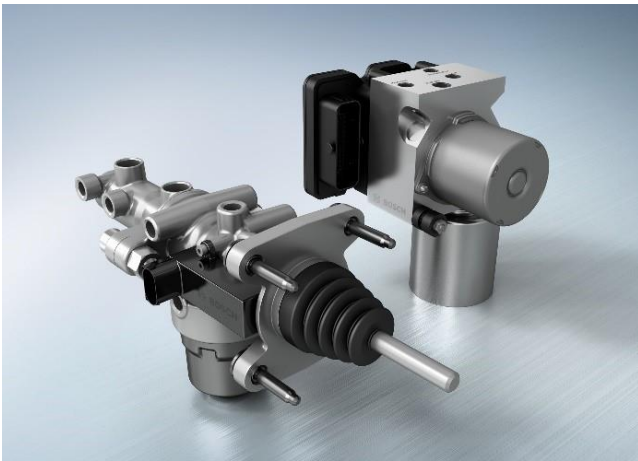
Figure 108 Vacuum-independent braking system specially designed for plug-in hybrids and electric vehicles. It comprises a brake operation unit (left) and an actuation control module (right) which supplement the ESP® hydraulic modulator (Source: Bosch Media)
