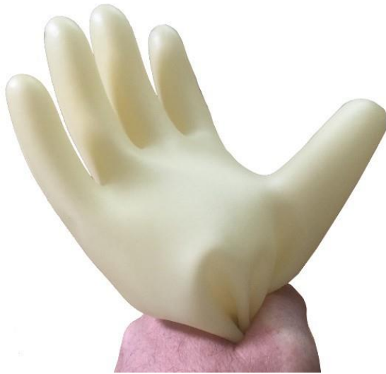
Figure 24 Electrical glove inflation test
