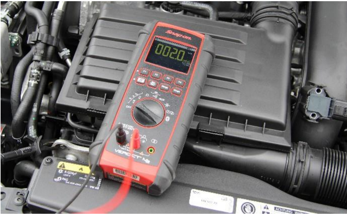
Figure 50. Ghost voltage caused by shaking the red lead
