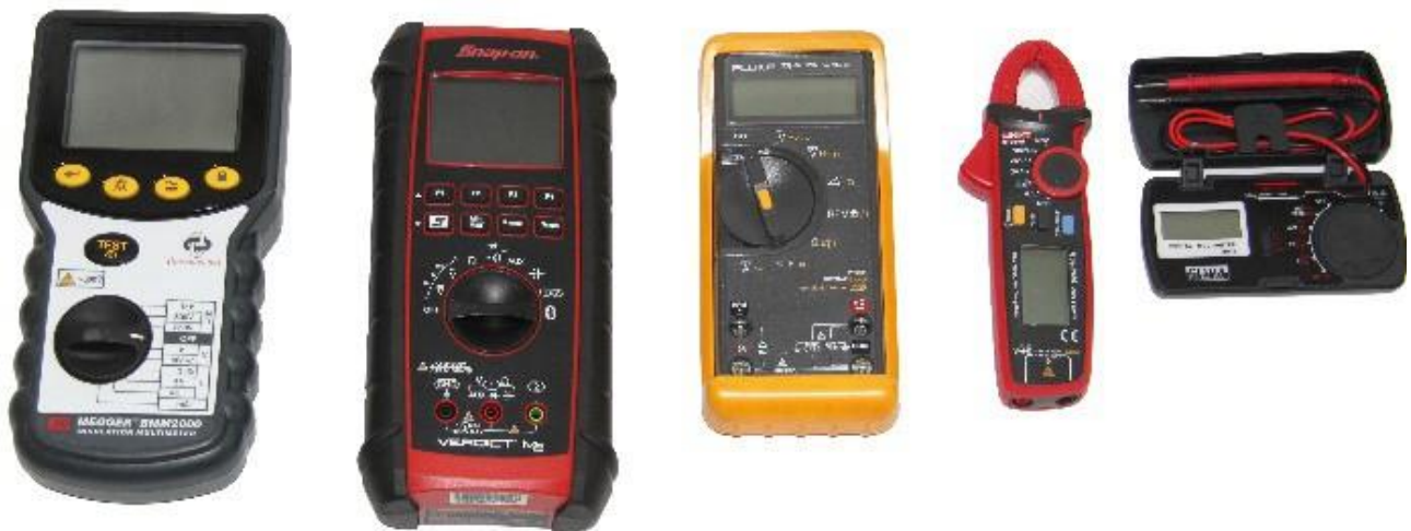
Figure 43 Multimeters (left to right): Megger insulation tester and meter, Snap-on Scope meter, Fluke 78 Automotive meter, Uni-T amp clamp meter and Sealey pocket meter
