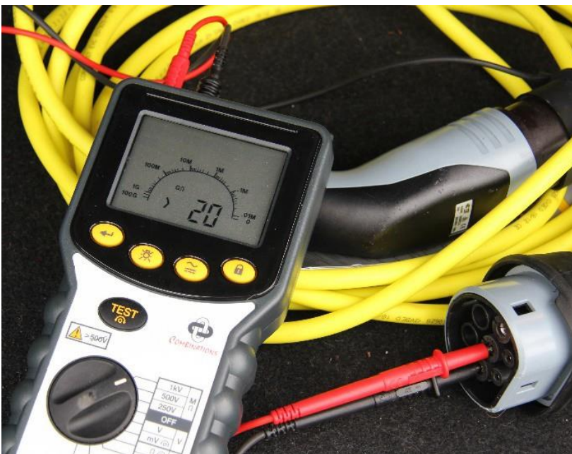
Figure 51. Checking the insulation resistance between conductors in an EV charging lead (in this case the reading is greater than 20GΩ)
