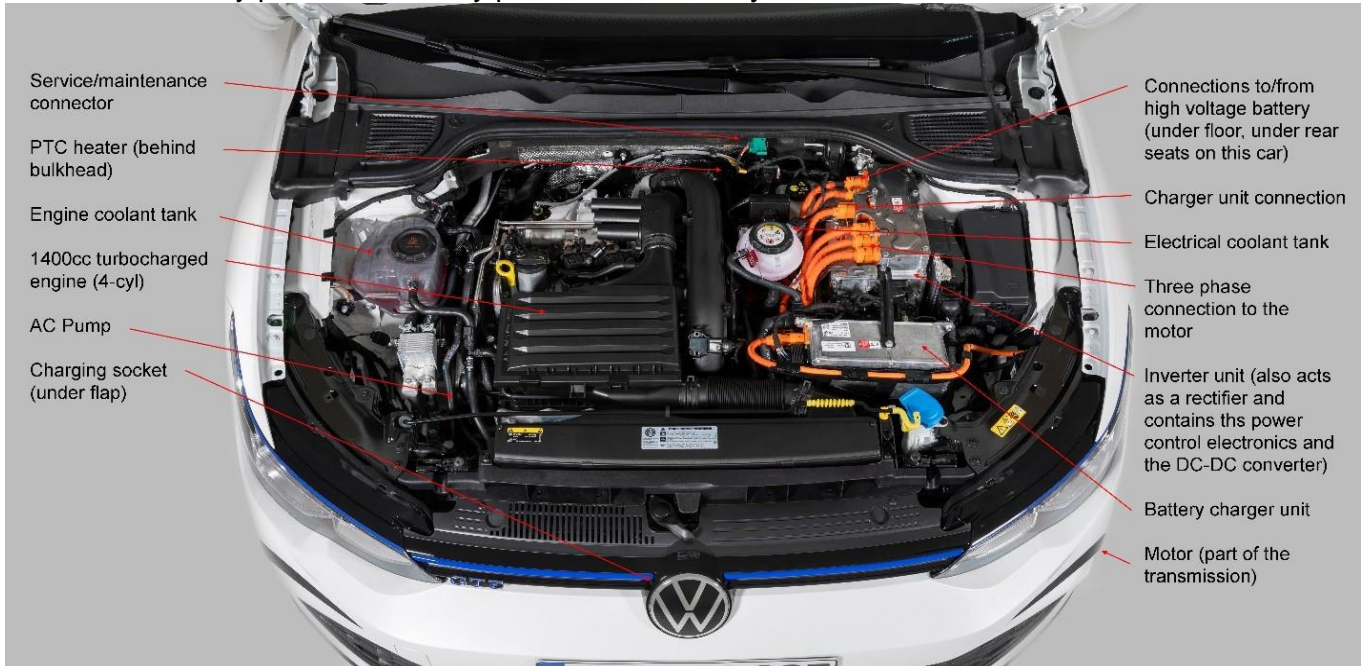
Figure 102 Plug-in hybrid car with components labeled (Source: Volkswagen Media)
