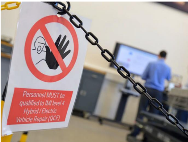
Figure 33 Work area fenced off and a warning sign in place
