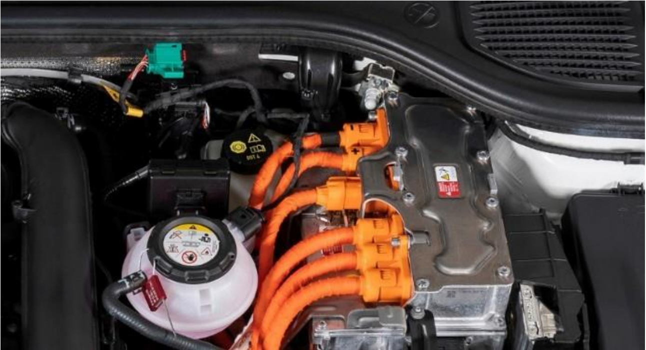
Figure 34 PHEV showing the maintenance connector (green component on the bulkhead)
