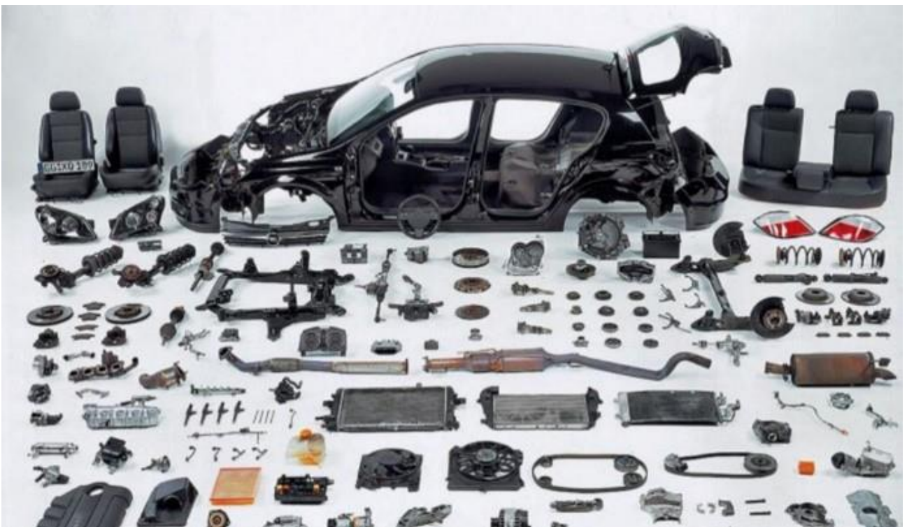
Figure 203 Example of components that can be reused. EV components are likely to have a much higher value
