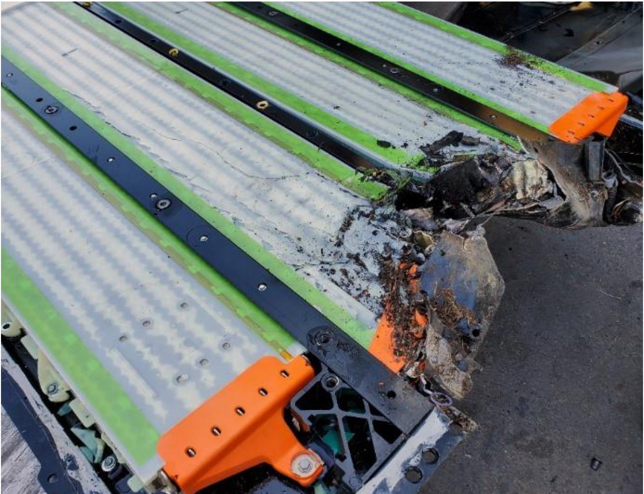
Figure 195 High voltage battery damaged during an accident
