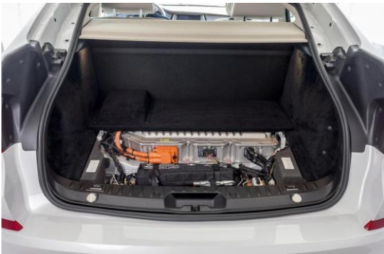
Figure 100 Battery cables (Source: BMW Media)
