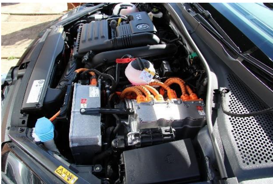
Figure 14 High voltage cables are always orange
