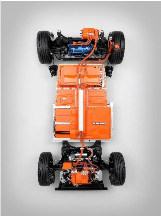
Figure 125 Battery pack and other HV components on the Volvo SUV (Source: Volvo Media)
