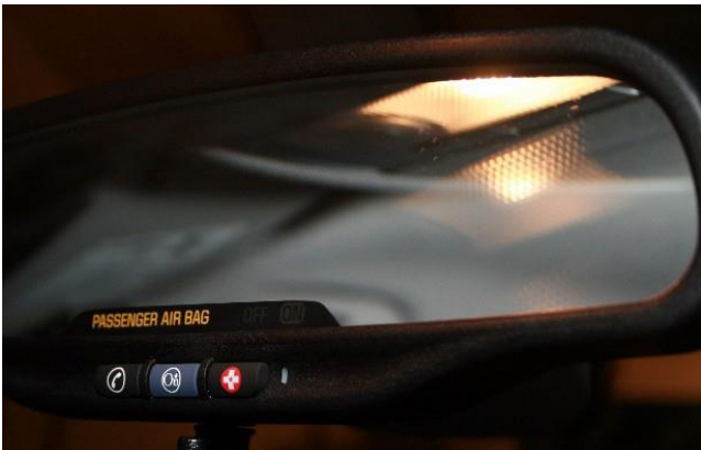
Figure 146 Access to emergency systems is usually by a button under the rear-view mirror
