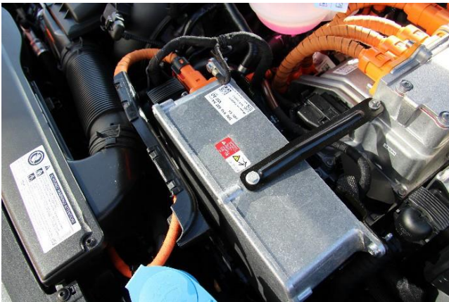
Figure 99 Orange cables and warning stickers on a Golf GTE
