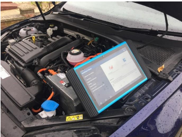
Figure 199 Electronic data can be accessed online using this diagnostic tool
