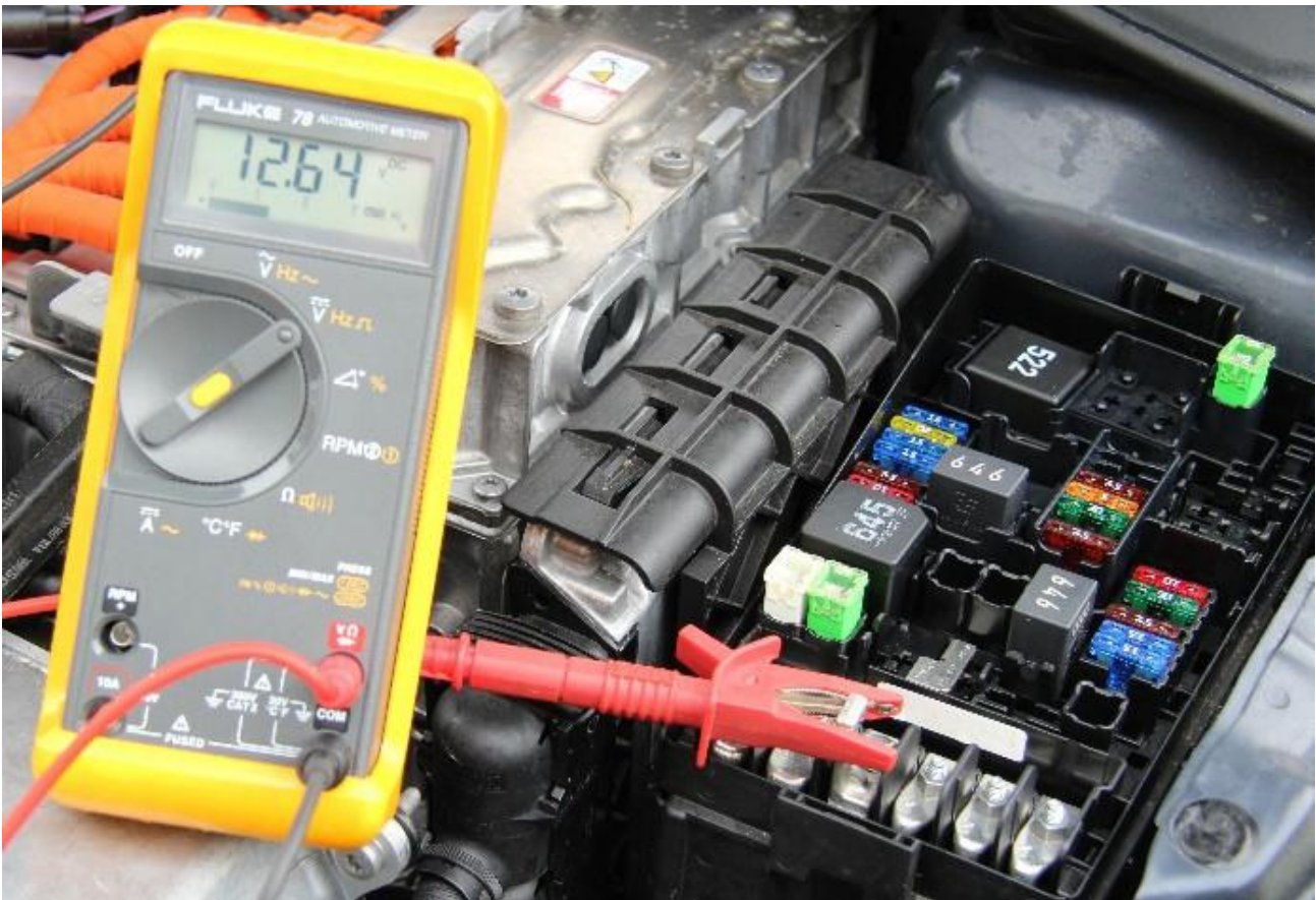
Figure 47. Voltage supply to a fuse box
