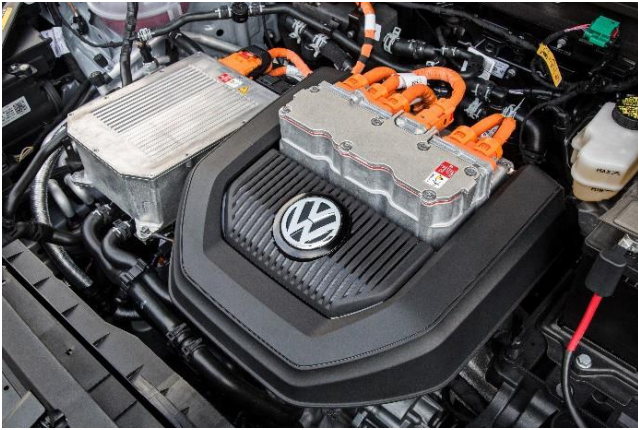
Figure 98 VW e-Golf showing some of the orange cables
