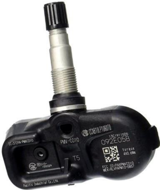
Figure 145 Some tire pressure sensors contain small mercury-based batteries.
