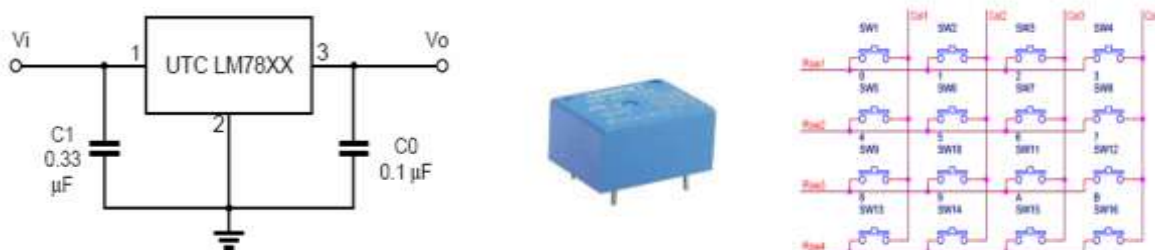
Fig.3: Voltage Regulator, Relay, Matrix keypad
