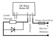
It is recommended to use a free wheeling diode connected in parallel with the load. Use connection wires as short as possible.
