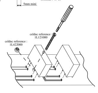
Warning! semiconductor relays don't provide any galvanic insulation between the load and the mains. Always use in conjunction with an adapted circuit breaker with isolation feature or a similar device in order to ensure a reliable isolation in the event of malfunction and when the relay must be insulated from the mains (maintenance; if not used for a long duration ...).
