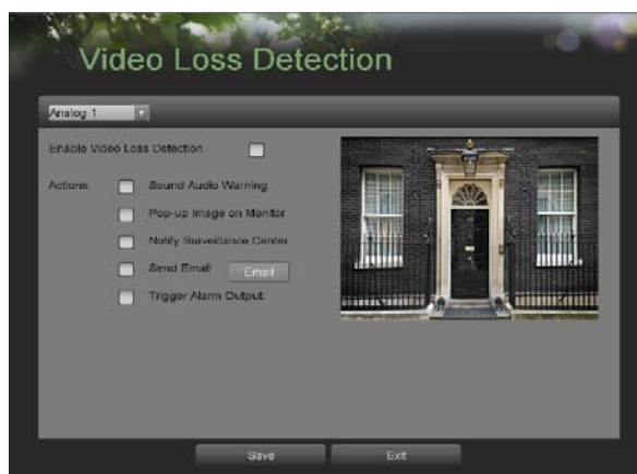
Figure 52. Video Loss Detection Menu
