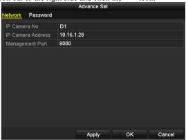
Figure 2. 25 Network Configuration of the Camera
