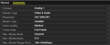
Figure 5. 55 Sub-stream Encoding
