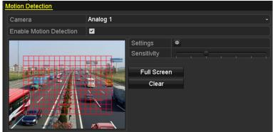
Figure 5. 63 Motion Detection- Mask
