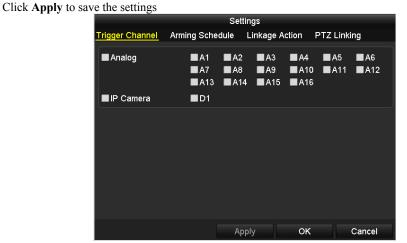
Figure 5. 70 Set Trigger Camera of VCA Alarm
