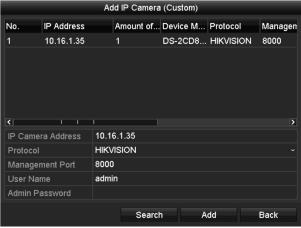
Figure 2. 20 Custom Adding IP Camera Interface
