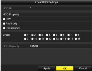
Figure 10. 200 Local HDD Settings Interface
