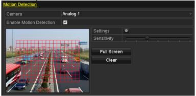
Figure 8. 127 Set Detection Area and Sensitivity
