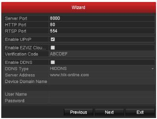
Figure 2. 15 Advanced Network Configuration
