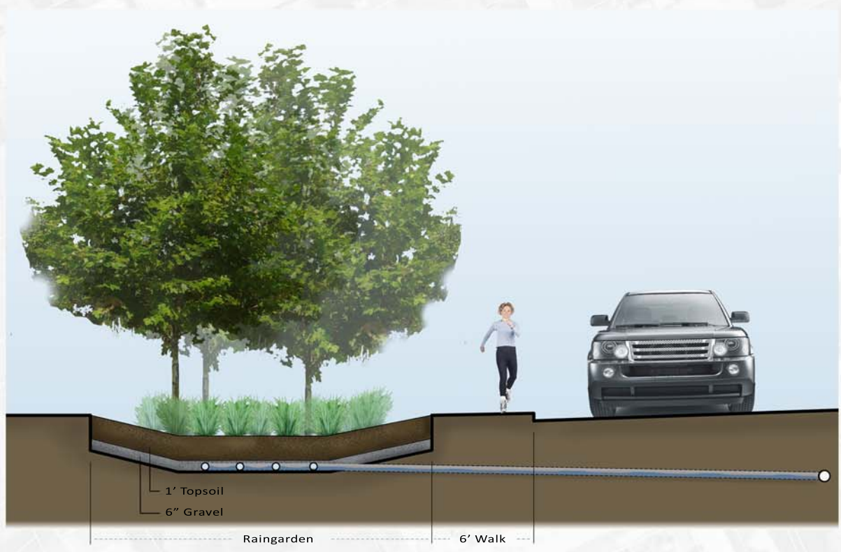
Raingarden With Underdrains
