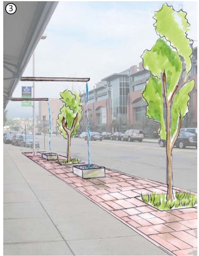
Even though storage units will be underground, the surface will be made of pervious pavers that do not take away from sidewalk space.
