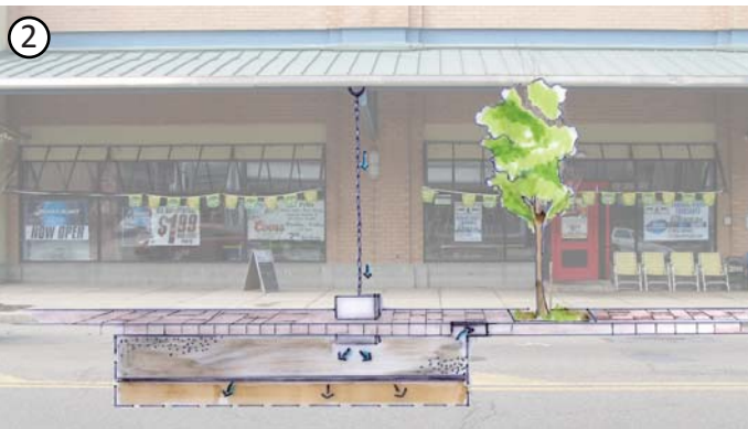
The water can be brought into catchment containers and given the opportunity to infiltrate through underground storage.
