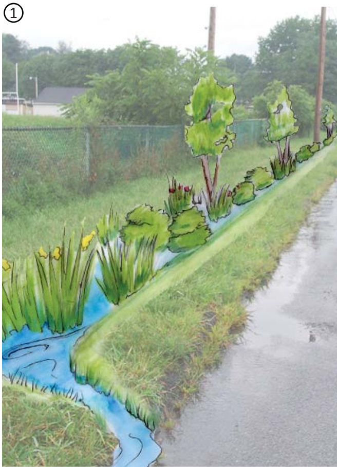
Approximately twelve feet of area between the edge of pave along Elm Street and the fence line create an ideal location to take water from the existing street gutter and direct it down a vegetated channel.
