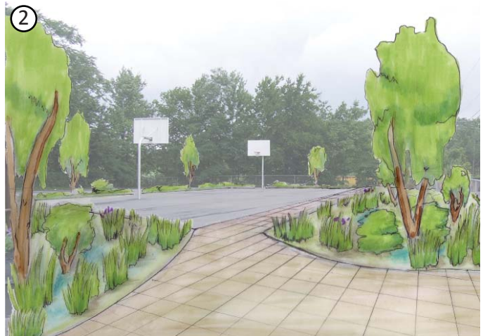
Asphalt surrounding the basketball courts can be converted into a vegetated swale that collects runoff and reduces overall impervious area. (approx. 6' wide)
