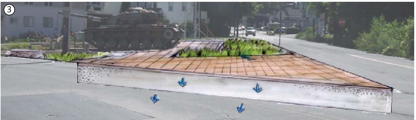
Existing asphalt triangle next to memorial will be converted to permeable paves with an infiltration pit under it to deal with excess water from rain gardens.
