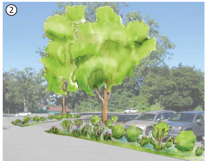
2 The parking lot on the north side of the park can be redesigned and implement a long rain garden to catch stormwater.
