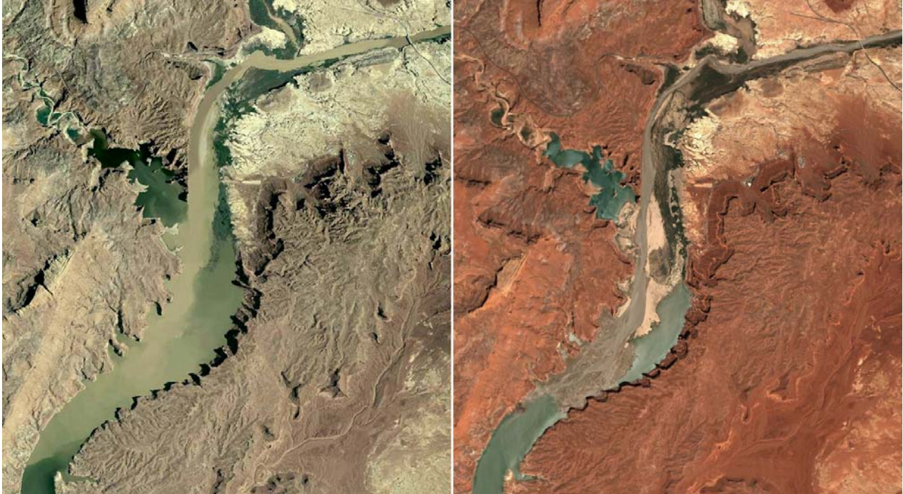
Left: Sediment-laden water from the Colorado River entering Lake Powell near the Hite Bridge. Right: Delta sediment deposits visible at the same location at a lower reservoir water level. (Satellite images obtained from Utah Automated Geographic Resource Center and Google Earth, 2008.)
