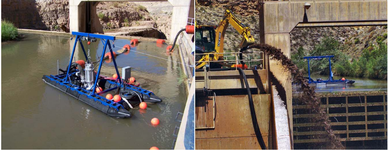
Hydraulic dredging device in operation at Quail Creek Diversion Dam, near Hurricane. (Photos courtesy of Washington County Water Conservancy District.)
