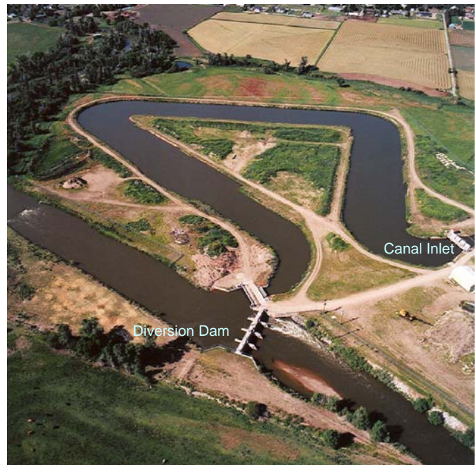
Aerial view of Stoddard Diversion Dam and the “meandering forebay” that serves as a sedimentation basin before water enters the canal. (Photo courtesy of Weber Basin Water Conservancy District.)
