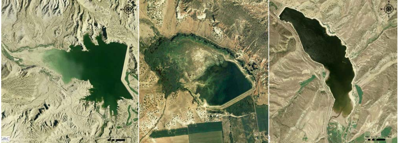
Left: Visible sediment deposits at Millsite Reservoir near Ferron.
