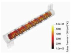
riangle Local heat transfer coefficient (Flow = 5  $m^3$ /hour).
