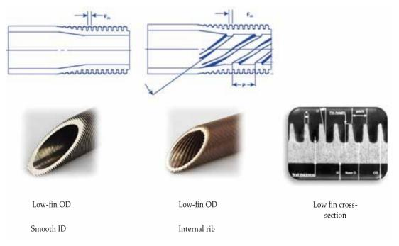
≈ Figure 1 : Illustration of low fins and internal ribs enhancements
