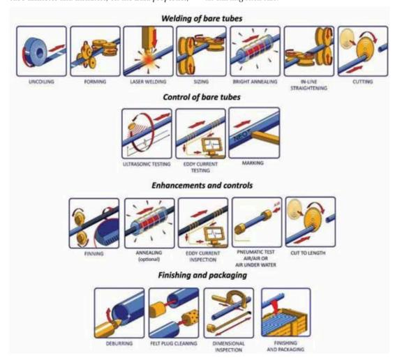
≈ Figure 3 : Example of process from the strip to ready-to-ship tubes
