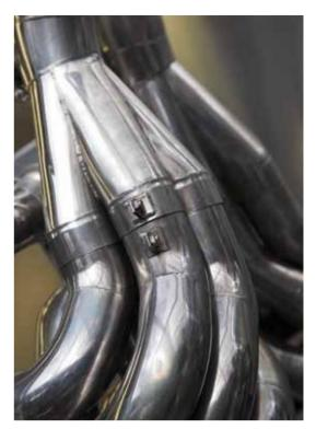
Stainless-steel exhaust system from a racing car.
