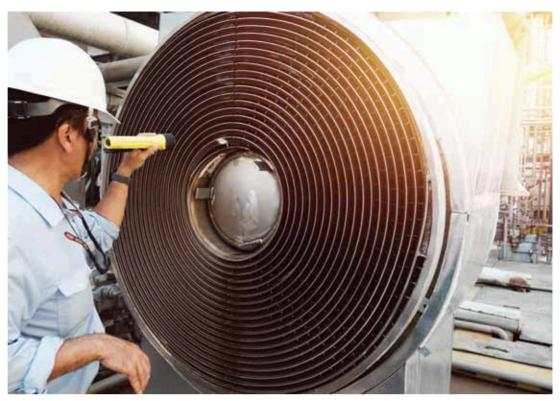
≈ Engineer inspects spiral heat exchanger in petroleum industrial plant.
