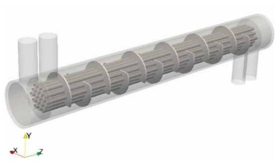
≈ Shell-and-tube heat exchanger geometry.
