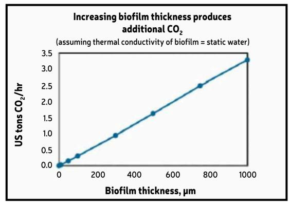
≈ Figure 1. The relationship between heat exchanger fouling and its environmental impact.
