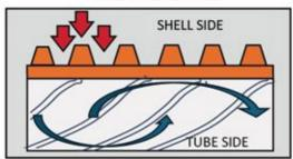
≈ Figure 2 : Increase in area and turbulent flow induced by dual enhanced tubes
