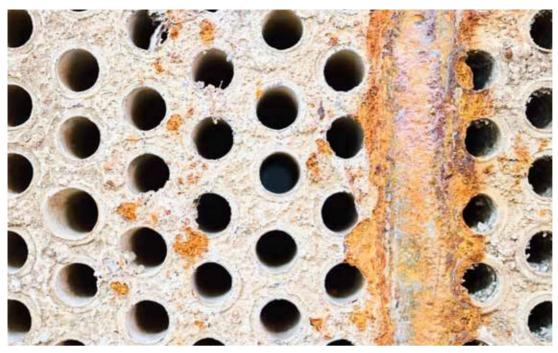
≈ Heat exchanger closeup full of hard insoluble mineral deposits, salts scale and corrosion.
