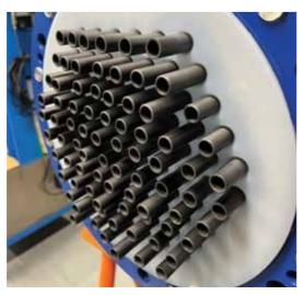
A Heat exchanger with SiC tubes.
