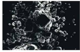
≈ Lime deposits in water treated with QMT Collar. Magnification 250x.
