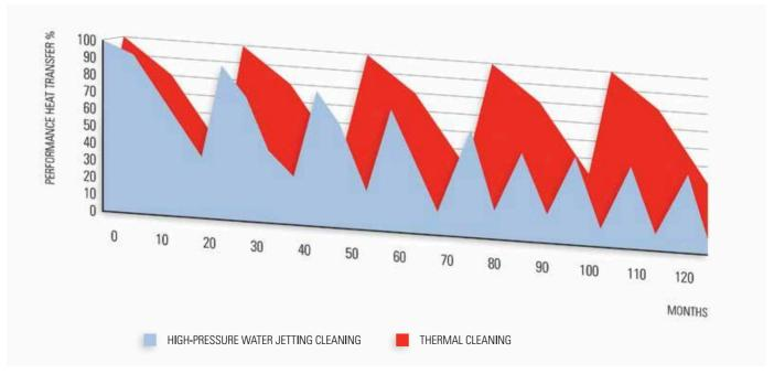
a Comparison of cleaning frequency high-pressure water jetting vs. thermal.
