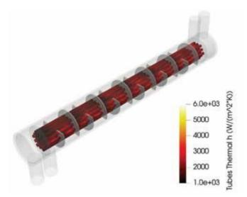
ightharpoonup Local heat transfer coefficient (Flow = 3 m³/hour).
