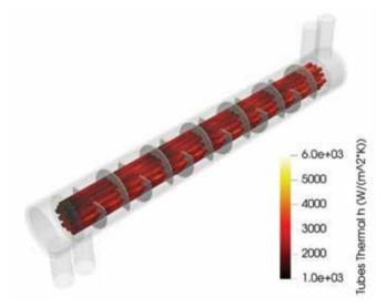
riangle Local heat transfer coefficient (Flow = 4 m³/hour).
