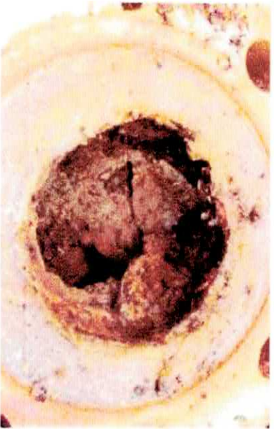
The pipe of exchanger without quantum ring
