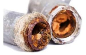
During the operation of the industrial circulation cooling process, there is a layer of metal oxide on the surface of the equipment and pipes.
