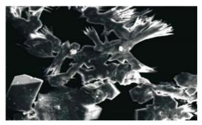
Lime deposits in untreated water. Magnification: 250x
