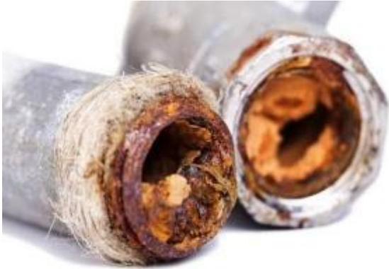
During the operation of the industrial circulation cooling process, there is a layer of metal oxide on the surface of the equipment and pipes.
