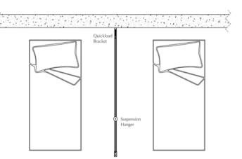
**Install Illustration:** Quickload Bracket attaches to wall, Suspension Hanger to ceiling
