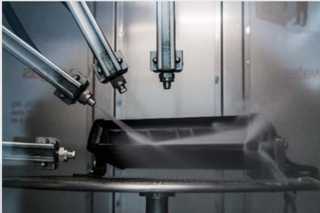
Water resistance Protection class IP6K8/ IP6K9K
