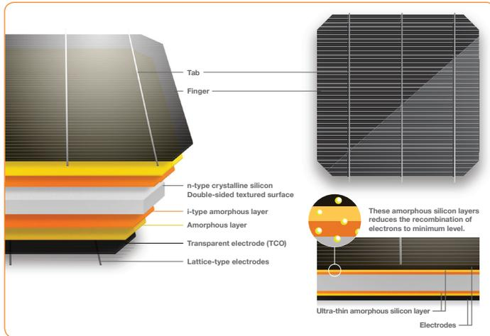
Advanced bifacial cell designed for increased energy output. The cell utilizes sunlight reflected back from the rear side material which captures more light and converted into energy.
