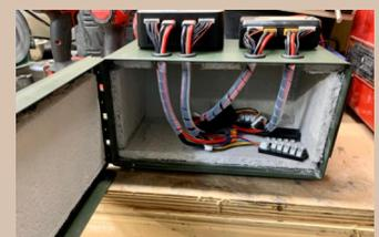
This picture shows how a fellow hobbyist turned a used ammo case into a Homemade battery firebox—lined with fireplace brick inserts..
