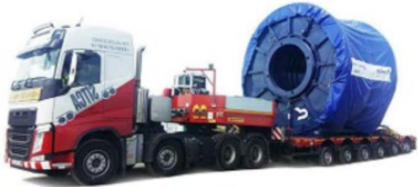
Low Loader (Cable Drum Delivery) Overall Length 25.440m
