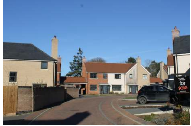
This high quality streetscene could be much improved by replacement of the high brick wall and close-boarded fence with a more appropriate boundary treatment (such as a hedge, low railing or low brick wall)
