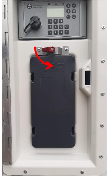
Figure 14 Retainer in de open position, turn counter clockwise to close
