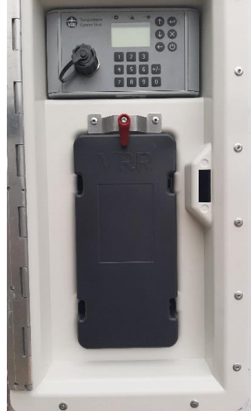
Figure 15 Retainer closed, turn clockwise to open
