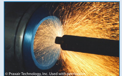
Wire arc coating is applied to the inside of a cylinder.
