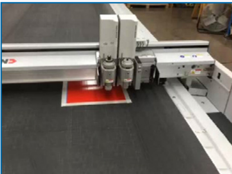
A CNC Plotter cuts repetitive shapes from a sheet of 170-105 Red plasma spray masking tape.
