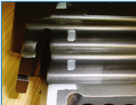
A part with recurring rectangular target areas is efficiently masked (left) with 170-10S Green HVOF tape with die-cut windows. The image on the right shows the part with masking removed, after receiving the spray coating.
