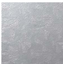
Acrylic Coated Galvalume TSR = 55%
