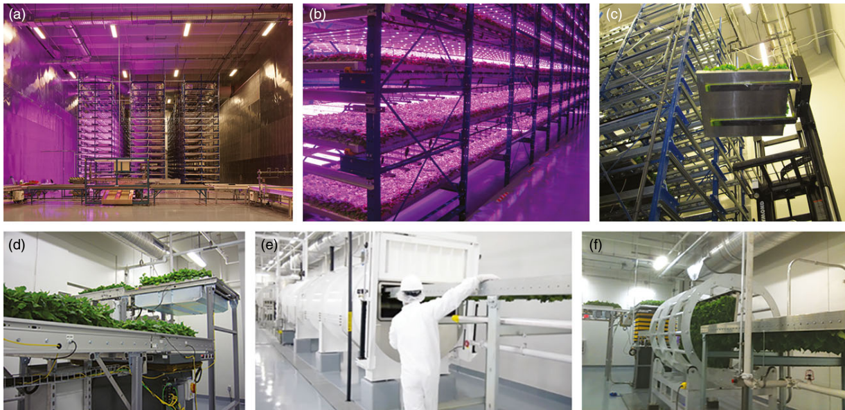
Figure 3 Illustration of semi-automated plant growth and infiltration procedure. (a) Germination room showing laminar flow walls, plant growth flow racks and the robotic transplanter (in the foreground); (b) N. benthamiana growing under LED lights in the germination room; (c) forklift operation for tray racking; (d) plant grow trays conveyed into the infiltration room; (e) plant trays entering custom-designed infiltrator; (f) plant trays exiting the infiltrator, inverted backup and conveyed to the postinfiltration rooms.
