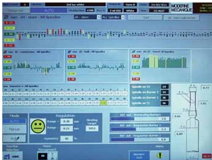
Main page of control panel with control of diameters trend and work of proportional valves in pre-heating burners
