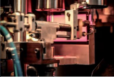
The CRM camera, which is installed in fix position, makes dimensional control of finished vials before unloading to the line. The control is made on all the main vial dimensions (except the total length) and neck eccentricity. According to these information out of tollerance vials are automatically rejected.
