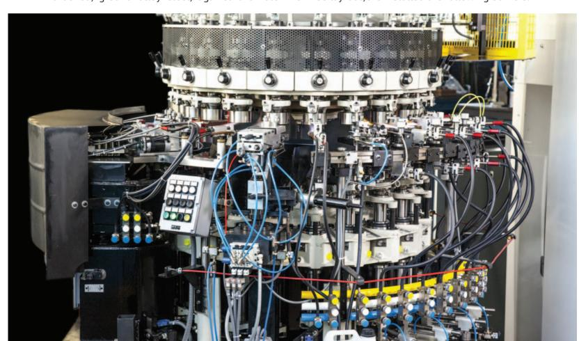
Pre-heating burners Bottom forming burners Final forming burners
