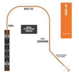
The standard traffic pattern consists of a downwind, base, and final leg. As the graphic shows, the downwind leg is parallel to the active runway and in the opposite direction of the landing. On this leg you will likely have a tailwind, assuming the wind is in the direction of the runway.
