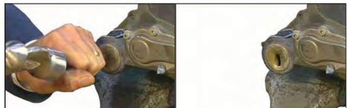
Figure 63 – Punch Guide Pin Cap (10)
