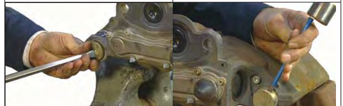
Figure 65 – Pry to Remove Guide Pin Cap (10)
