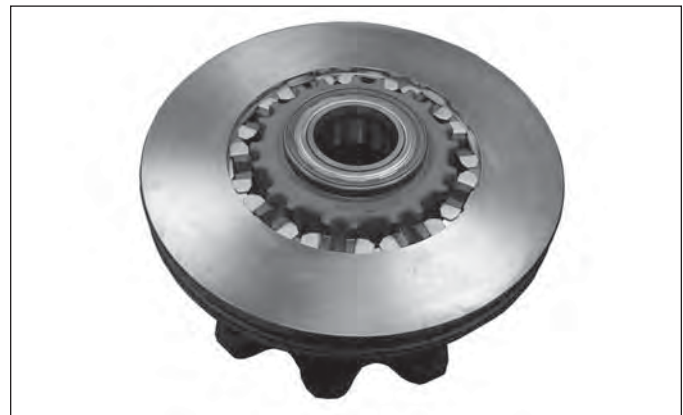
Figure 90 – Intermediate Elements (Spacers) Installed
