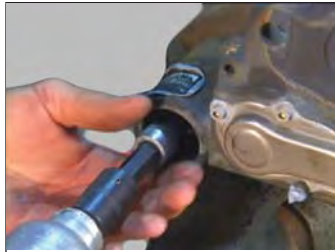
Figure 67 – Remove the Caliper Bolts
