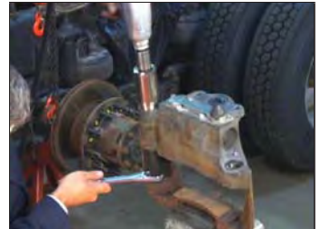
Figure 71 – Remove the Long Guide Pin
