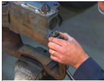
Figure 78 – Position the New Bushing
