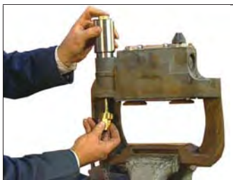
Figure 70 – Install the Removal Tool
