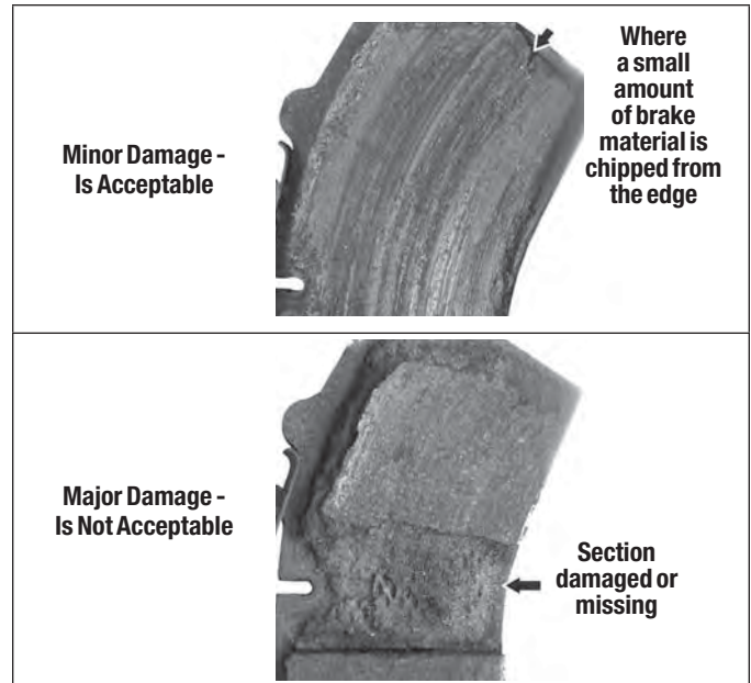
Figure 24 – Brake Pad Surface Inspection
