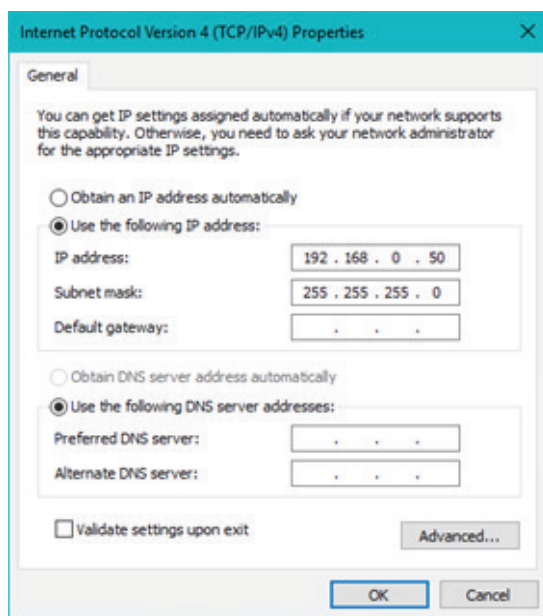
Figure 25: Internet Protocol Version 4 (TCP/IPv4) Properties Customization
