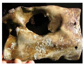
Cover of one of the 2 propeller relay box. This relay box was under the engine. One can see a big hole, certainly done by one of the numerous shell sent through the air by the bomb mistakenlly launched by LTt Donald Erickson
