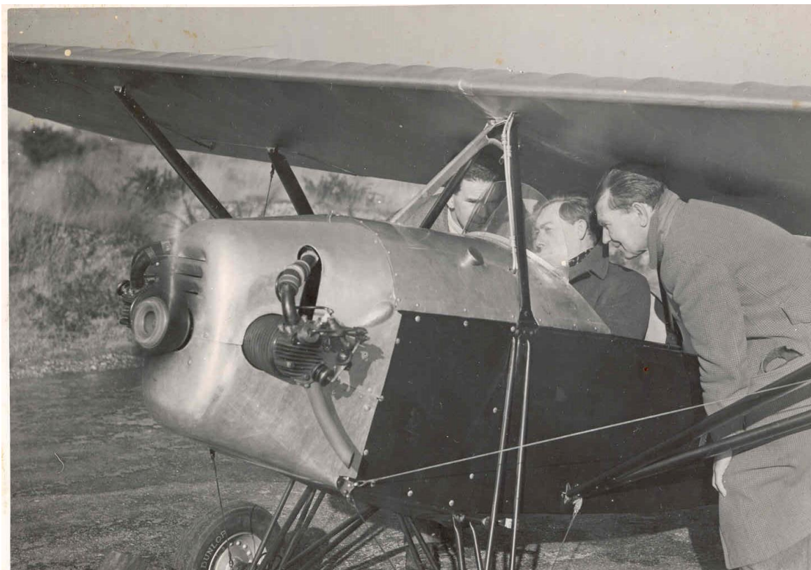
Heath Parasol G-AJCK with ABC engine at Christchurch. The Heath Parasol is an American single-seat, open-cockpit, parasol winged, homebuilt monoplane. During the late 1920s and early 1930s it was the only airplane in the USA that could be constructed at home from a factory-built kit and be licensed by the FAA. Seen below with Ron Clear in cockpit prior to first flight SHULAC secretary Bob Haigh on right.
