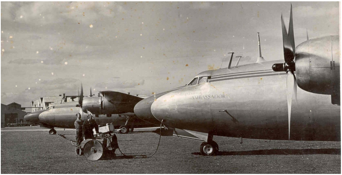
The two prototype Ambassadors being prepared for flight. The second prototype, which was pressurised, is in the background
