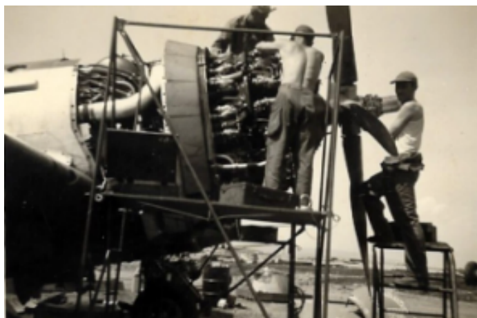
Engine change or engine maintenance of a P-47 of the 394th FS. Note the 2 rows of cylinders (Linda Tjepkes/archives 367 th FG)
